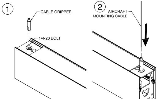
1. INSTALL ADJUSTABLE CABLE GRIPPER ON 1/4-20 **BOLT ON FIXTURE**
