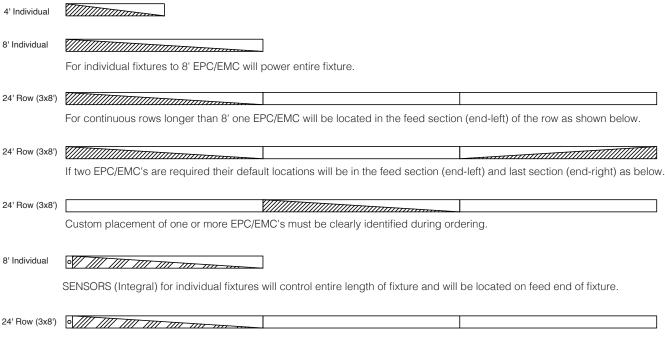
SENSORS for rows by default will control the feed section (end-left) of the row. Sensors can control more than an 8' section within a row. Consult factory for sensor/section options, or for multiple sensors in a continuous row.
