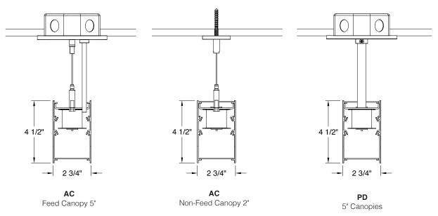
**AC-PF** = Replacement Power Feed Kit w/5" canopy. AC-NF = Replacement Non/Feed Kit w/2" canopy. Consult factory for custom lengths and either 5 or 6 wire power feeds.
