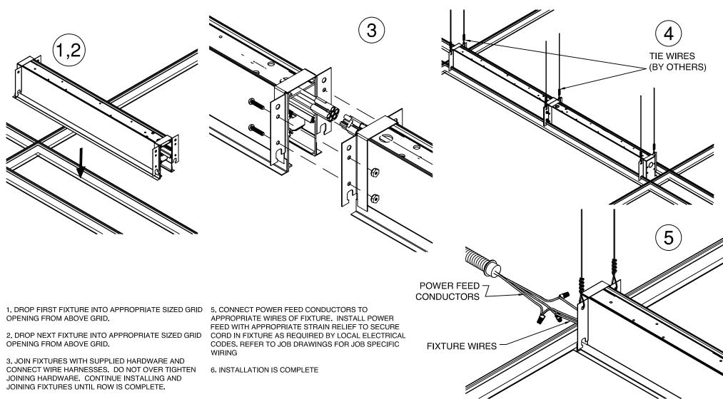
4. INSTALL TIE WIRE TO FIXTURE AND SECURE OTHER END TO APPROPRIATE STRUCTURE TO SUPPORT
